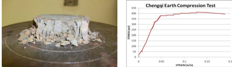
Figure 5: Chengqi earth sample after compression testing and resulting stress/strain curve
