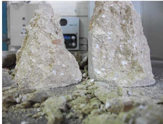
Figure 4: Batch 5 sample after being tested to measure the unconfined compressive strength (UCS). The white particles represent the intact perlite grains.
