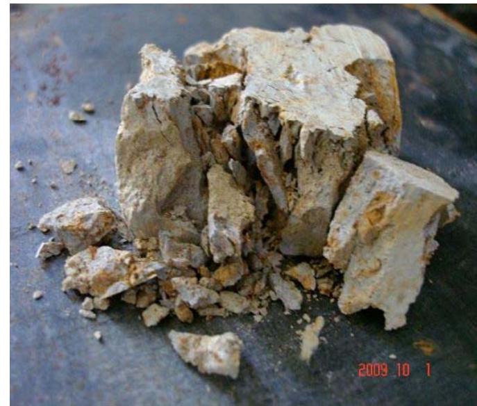
Failed rammed earth sample (XMU)
