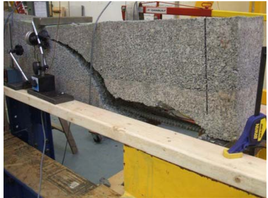
Flexural Capacity Achieved
