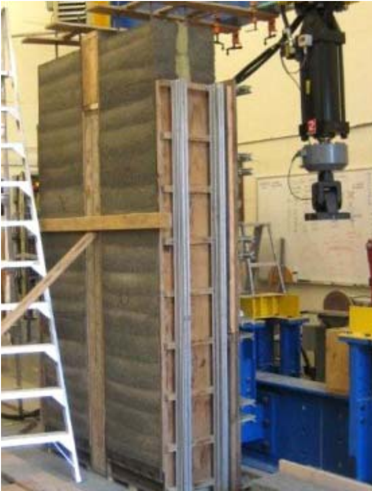
Wall Columns – Forms Removed
