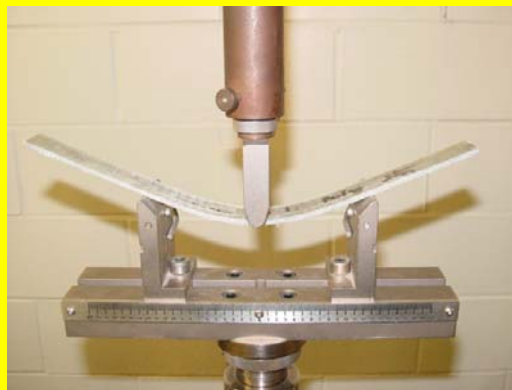
Three Point Bending Test ASTM D-790
